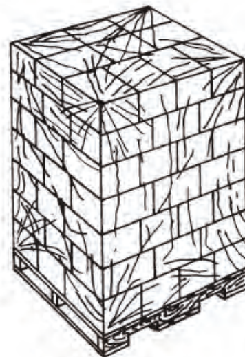
Pallet Load Utilizing One of the Stretch Wrap or Shrink-Wrapping Films
